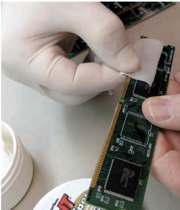
Figure 4: Deoxidizing the board
