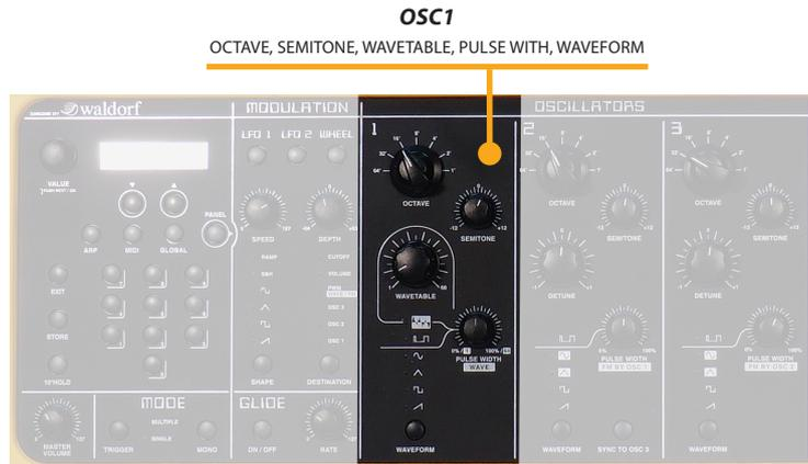
**Octave:** the range is from 64' to 1' (7 octaves); please note that the standard range for a piano is 8' and this means that, by setting the related control to the middle position, any key played on the keyboard will play with the same frequency of a standard piano (the Sledge keyboard is from C2 to C7 while the standard 88 notes piano range is from A0 to C8)
