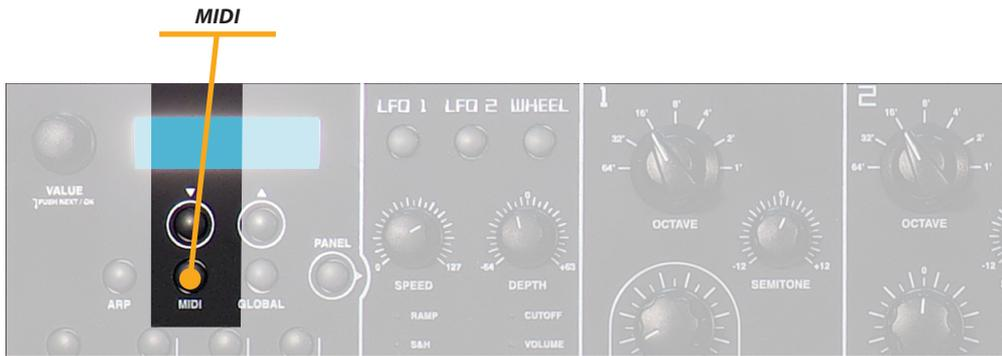
**MIDI** The Midi controls are related to all Midi Interface functions of the Sledge, allowing it to control external units and/or to be controlled by external units. The related pages (scrolled by the navigation tabs under the display) are:
