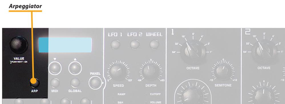
This function is a real-time automatic arpeggio generator, under control of few, clear and simple user's programmable menu pages, that can be scrolled by the dedicated buttons under the display while the desired control and/or parameter is selected by rotating the Value encoder.
