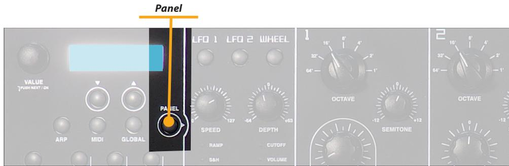
**Panel** This control allows to read at once all potentiometers physical position and generate all related controls on the various parameters, to instantly align the sound generation to the control panel.
